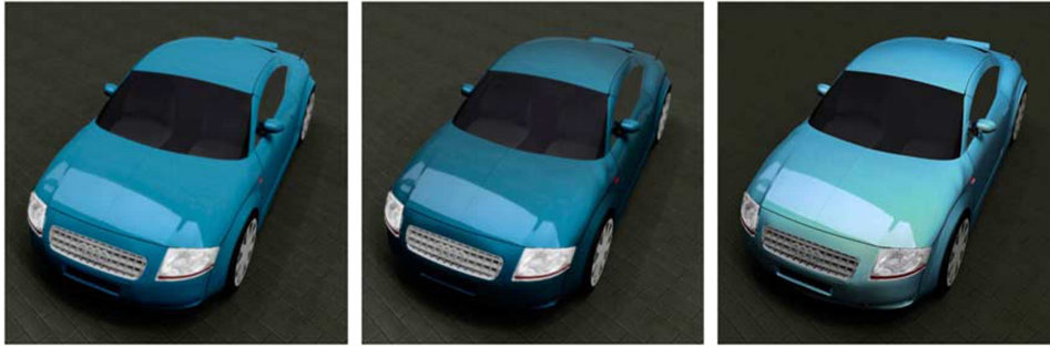
Figure 5.1: Cars with different coatings. Blue pigment only, added metallic flakes, added pearlescent flakes, respectively. Rendered using model 4.3 in paper [ĎÁ07]
