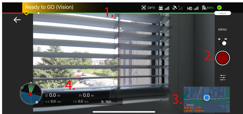
Figure 3.3: Drone Control View Screenshot – This image showcases the customized, versatile library component provided by the DJI SDK, illustrating the user interface used for detailed UAV control and adjustments.
